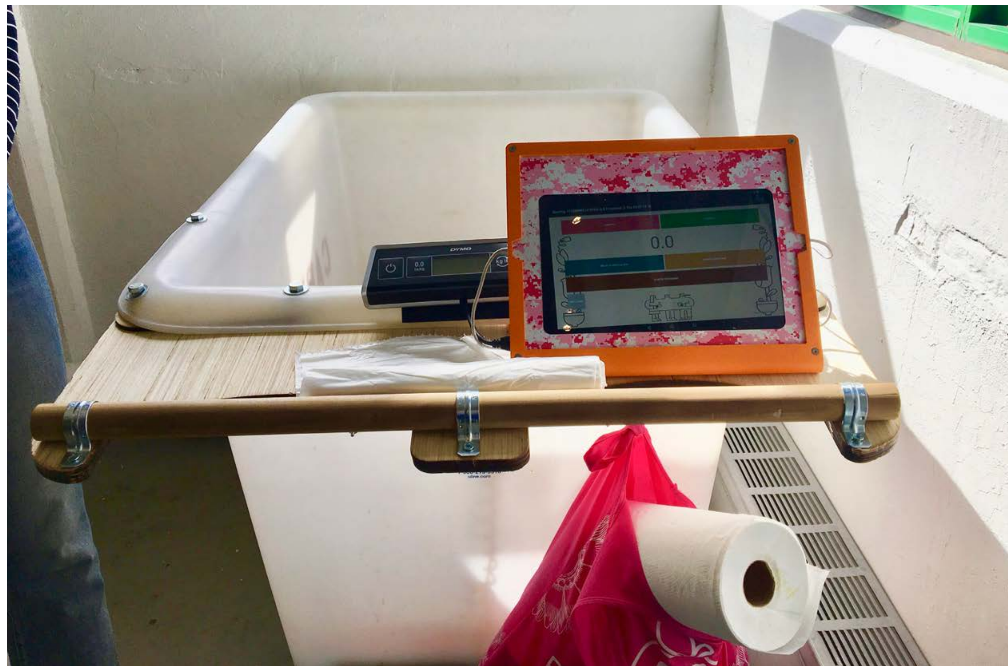
This is done by ensuring the cleaning staff use a hamper with scales and a tablet to record waste streams.
