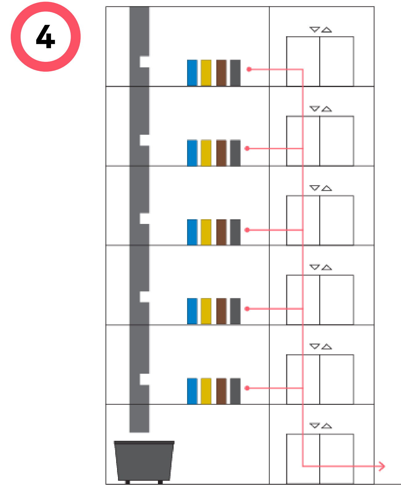
REFUSE ROOM WITH TRASH CHUTE AND RECYCLING BINS
