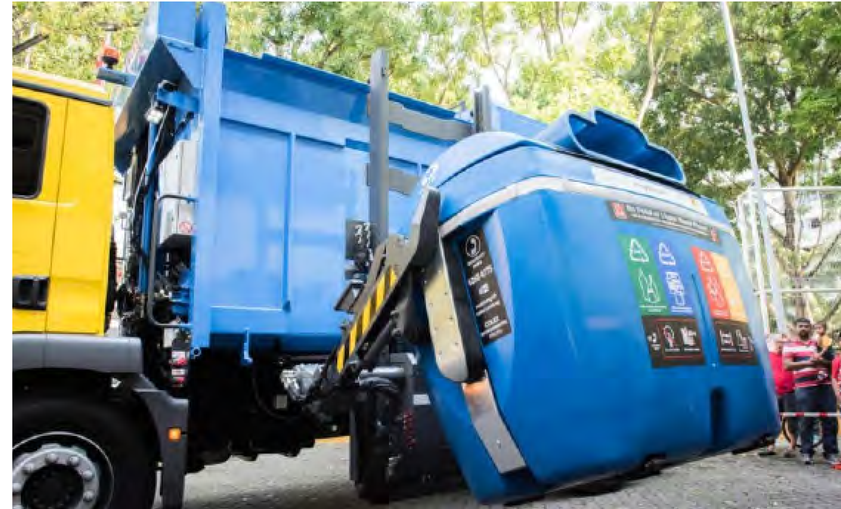
An automated side-loader recycling truck can lift larger 1200 and 2400 liter recycling bins.
