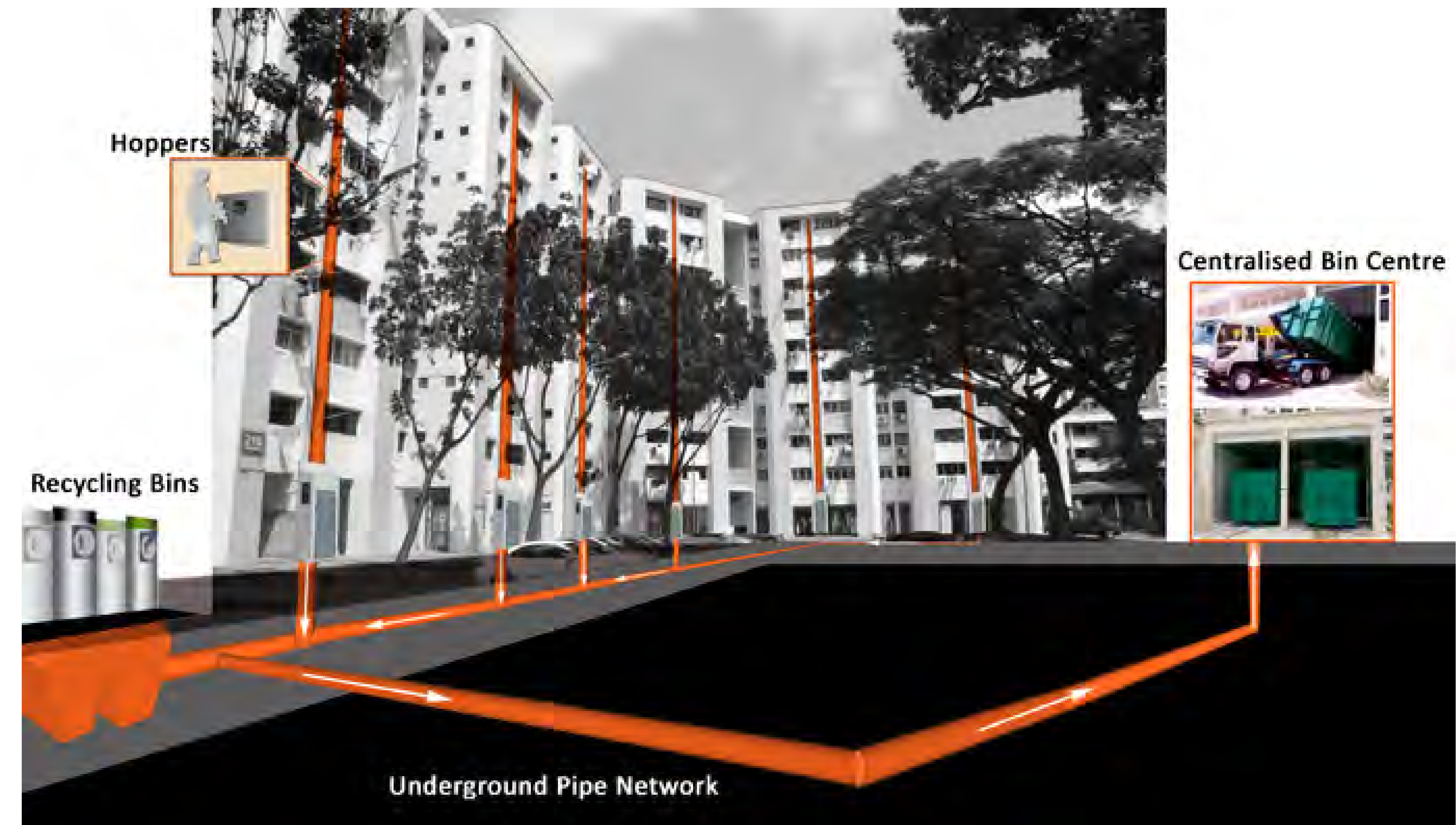
Pneumatic waste conveyance system at Yuhua.
