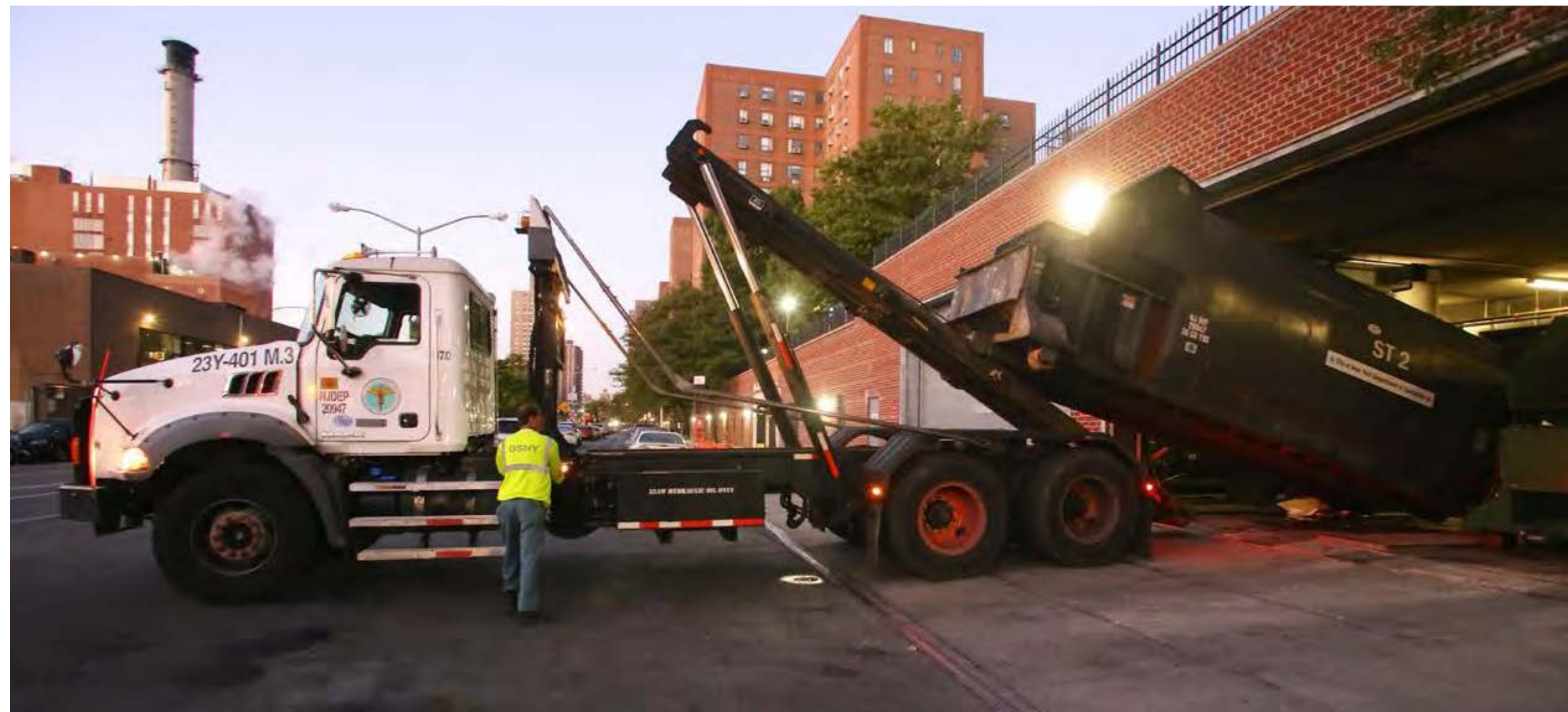
A RoRo container in the Stuy Town housing development. Current requirements for headroom are much higher than this installation
