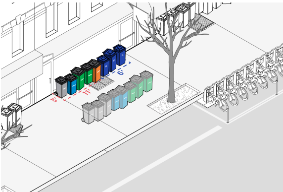
A 9 unit building will require \pm 13 bins for residences plus additional bins for the storefront business, exceeding the permitted 3 ft zone.
