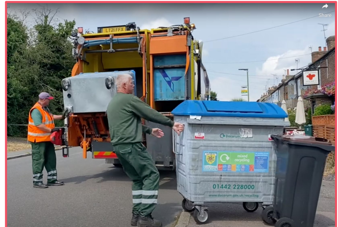
CfZWD’s solution will require porters from a 100 unit building to roll 4 wheeled bins (1100 liter = 1.4 cubic yard) to the street twice a week. This is much easier and more ergonomic for building staff.
